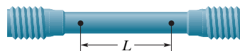
Fig. 12-11 A test specimen used to determine a stress–strain curve such as that of Fig. 12-12. The change \Delta L that occurs in a certain length L is measured in a tensile stress–strain test.
