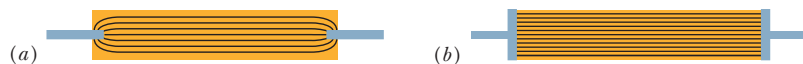
Fig. 26-8 Two ways of applying a potential difference to a conducting rod. The gray connectors are assumed to have negligible resistance. When they are arranged as in (a) in a small region at each rod end, the measured resistance is larger than when they are arranged as in (b) to cover the entire rod end.
