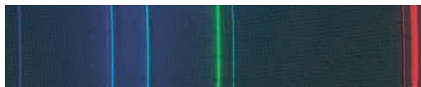
Fig. 36-25 The visible emission lines of cadmium, as seen through a grating spectroscopy. (Department of Physics, Imperial College/Science Photo Library/Photo Researchers)
