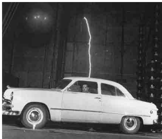
Fig. 24-19 A large spark jumps to a car's body and then exits by moving across the insulating left front tire (note the flash there), leaving the person inside unharmed. (Courtesy Westinghouse Electric Corporation)
