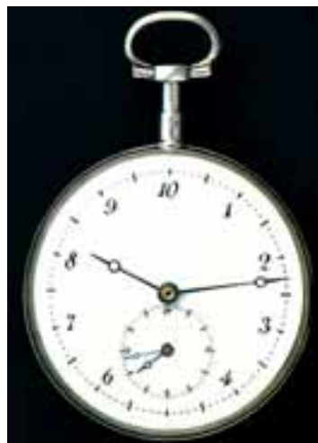
Fig. 1-1 When the metric system was proposed in 1792, the hour was redefined to provide a 10-hour day. The idea did not catch on. The maker of this 10-hour watch wisely provided a small dial that kept conventional 12-hour time. Do the two dials indicate the same time? (Steven Pitkin)
