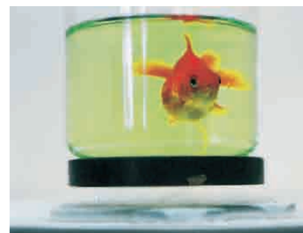
A disk-shaped magnet is levitated above a superconducting material that has been cooled by liquid nitrogen. The goldfish is along for the ride. (Courtesy Shoji Tonaka/International Superconductivity Technology Center, Tokyo, Japan)
