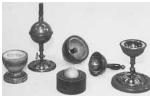
Fig. 25-12 The simple electrostatic apparatus used by Faraday. An assembled apparatus (second from left) forms a spherical capacitor consisting of a central brass ball and a concentric brass shell. Faraday placed dielectric materials in the space between the ball and the shell. ( The Royal Institute, England/Bridgeman Art Library/NY )
