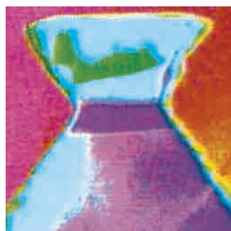
Fig. 39-11 A quantum dot, or “artificial atom.” (a) A central semiconducting layer forms a potential energy well in which electrons are trapped. The lower insulating layer is thin enough to allow electrons to be added to or removed from the central layer by barrier tunneling if an appropriate voltage is applied between the leads. (b) A photograph of an actual quantum dot. The central purple band is the electron confinement region. (From Scientific American , September 1995, page 67. Image reproduced with permission of H. Temkin, Texas Tech University)
